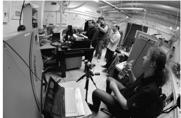
Figure 2 – Comparative spectroscopy in the laboratory of the J. Heyrovsky Institute of Physical Chemistry (the Czech Academy of Sciences) – the Echelle ESA 4000 high resolution spectrograph and the astronomical spectrograph QHY5LII-M.
