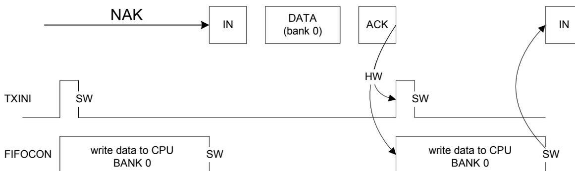
Figure 30-18. Example of an IN Endpoint with 2 Data Banks
