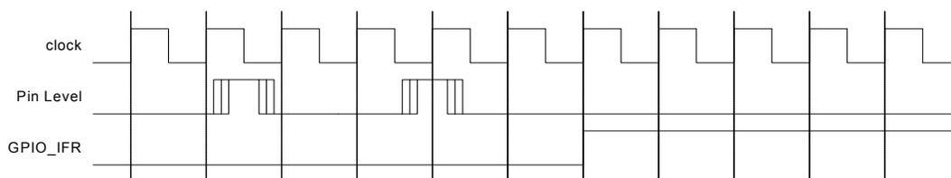
The figure below shows the timing for rising edge (or pin-change) interrupts when the glitch filter is enabled. For the pulse to be registered, it must be sampled on two subsequent rising edges. In the example, the first pulse is rejected while the second pulse is accepted and causes an interrupt request.
