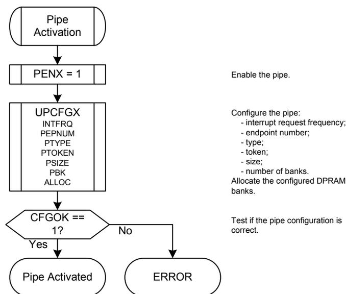
As long as the pipe is not correctly configured (CFGOK = 0), the controller can not send packets to the device through this pipe.
