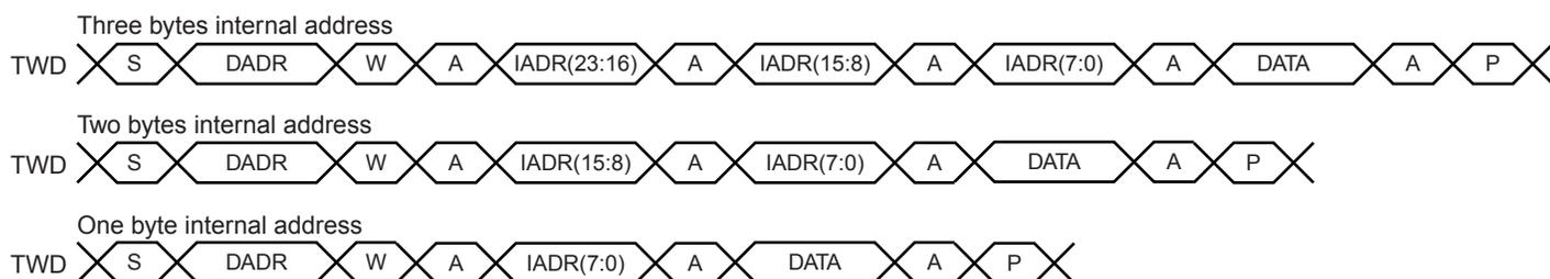
**Figure 24-12. Master Read with One, Two or Three Bytes Internal Address and One Data Byte**
