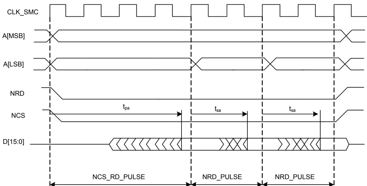
The NRD and NCS signals are held low during all read transfers, whatever the programmed values of the setup and hold timings in the User Interface may be. Moreover, the NRD and NCS timings are identical. The pulse length of the first access to the page is defined with the NCS\_RD\_PULSE field of the PULSE register. The pulse length of subsequent accesses within the page are defined using the NRD\_PULSE parameter.
