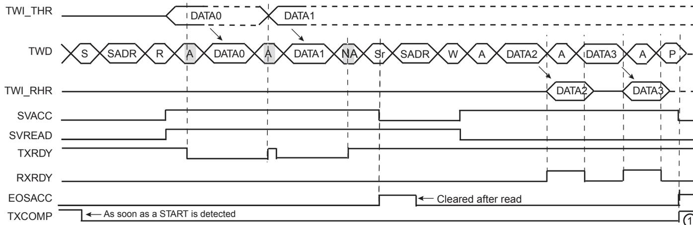
1. TXCOMP is only set at the end of the transmission because after the repeated start, SADR is detected again.
