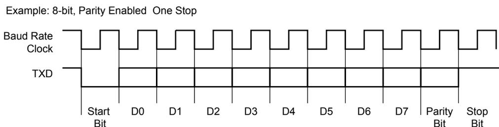
The characters are sent by writing in the Transmit Holding Register (THR). The transmitter reports two status bits in the Channel Status Register (CSR): TXRDY (Transmitter Ready), which indicates that THR is empty and TXEMPTY, which indicates that all the characters written in THR have been processed. When the current character processing is completed, the last character written in THR is transferred into the Shift Register of the transmitter and THR becomes empty, thus TXRDY rises.
