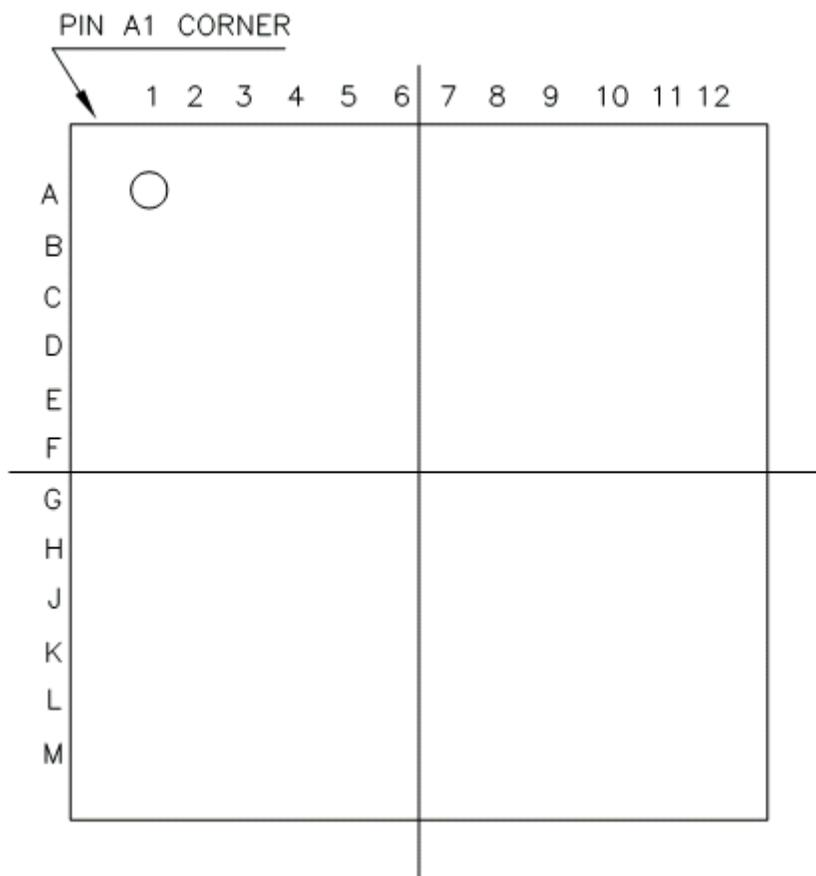
**Table 7-3.** BGA144 Package Pinout A1..M8
