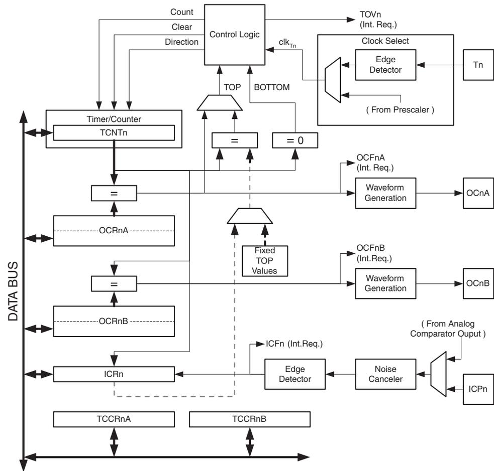
Note: 1. Refer to “Pin Configurations” on page 2, Table 22 on page 58, and Table 28 on page 63 for Timer/Counter1 pin placement and description.
