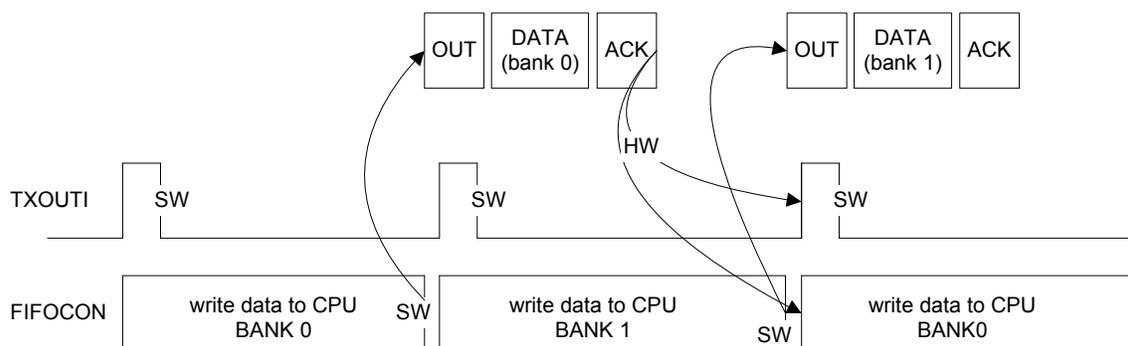
Figure 30-29. Example of an OUT Pipe with 2 Data Banks and a Bank Switching Delay
