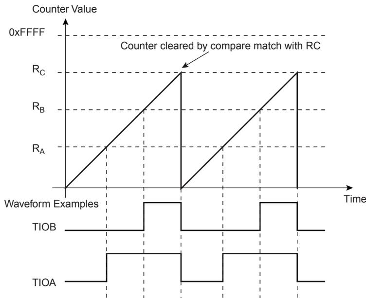
**Figure 31-9.** WAVSEL = 10 With Trigger
