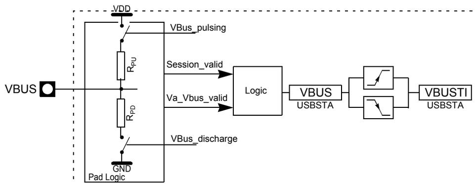
The control logic of the VBUS pad outputs two signals:
