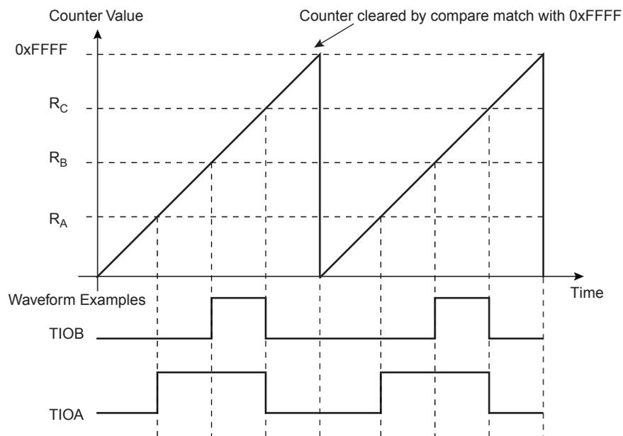
**Figure 31-7.** WAVSEL= 00 with trigger
