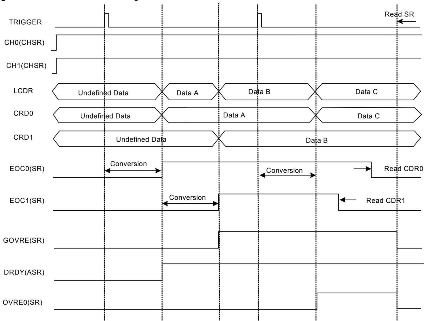
**Warning:** If the corresponding channel is disabled during a conversion or if it is disabled and then reenabled during a conversion, its associated data and its corresponding EOC and OVRE flags in SR are unpredictable.
