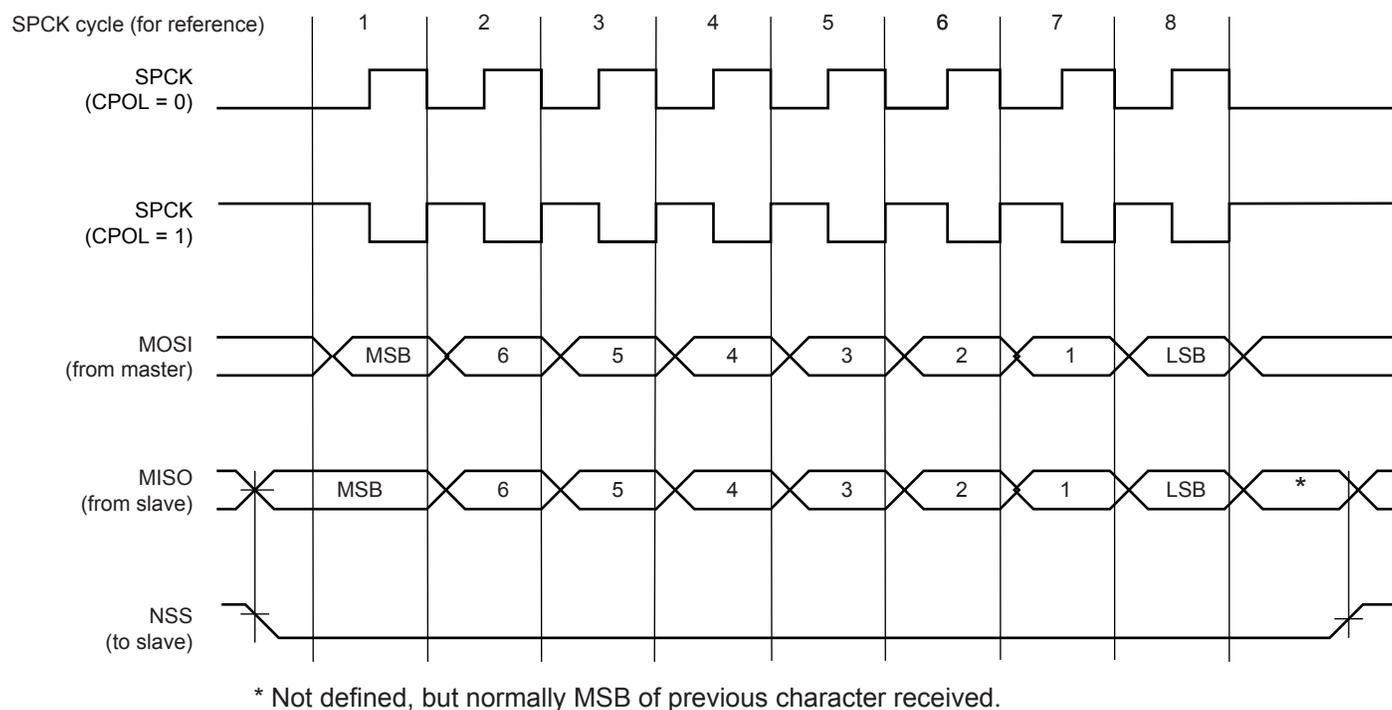
**Figure 23-4.** SPI Transfer Format (NCPHA = 0, 8 bits per transfer)
