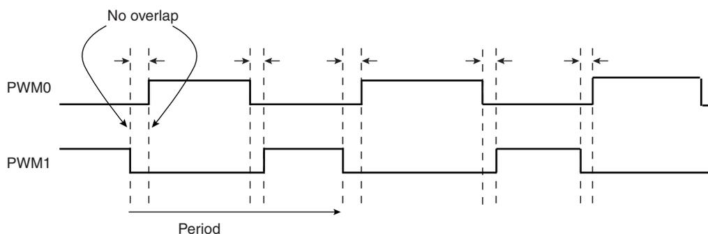
Note: 1. See [Figure 32-5 on page 680](#) for a detailed description of center aligned waveforms. When center aligned, the internal channel counter increases up to CPRD and decreases down to 0. This ends the period.
