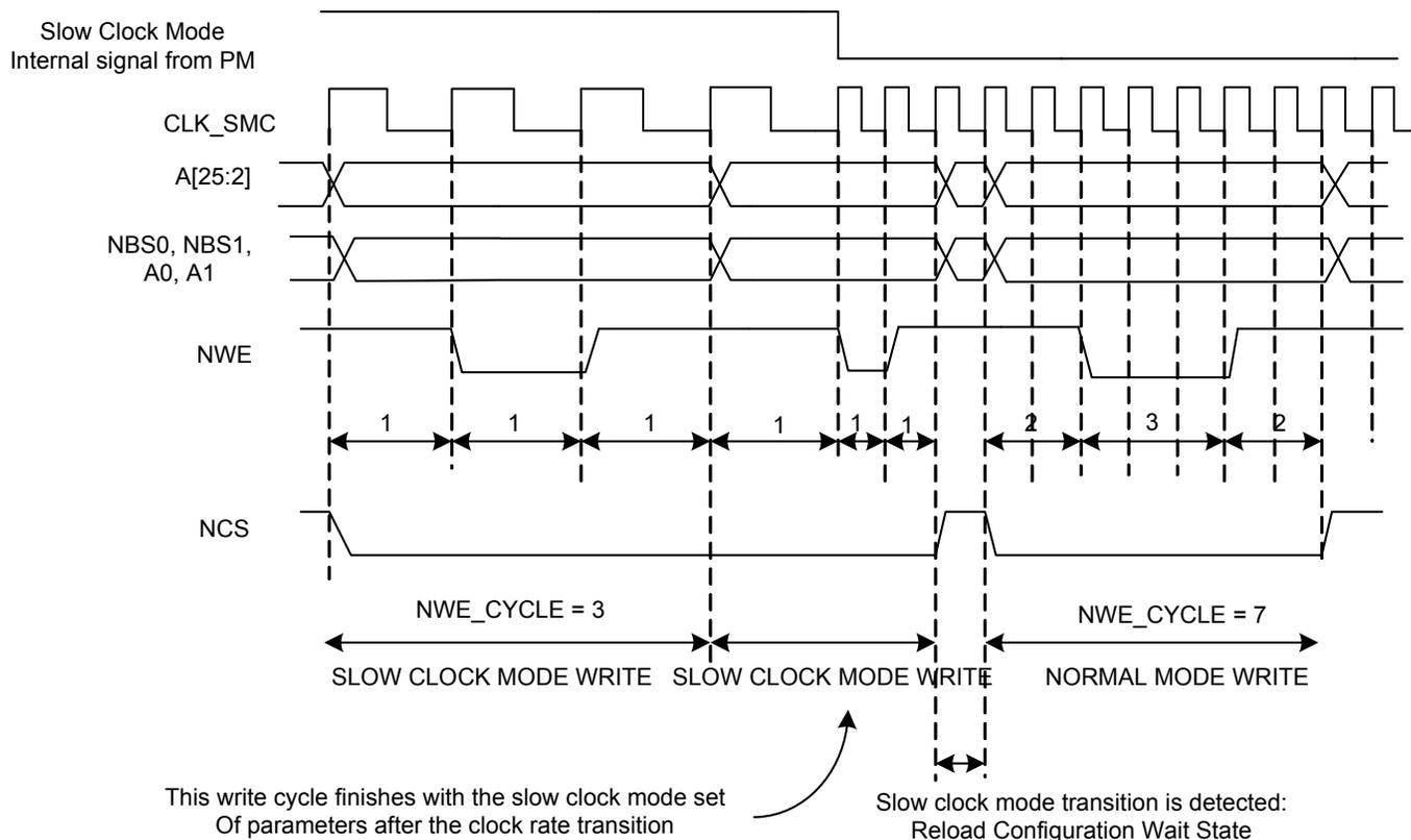
**Figure 27-34.** Recommended Procedure to Switch from Slow Clock Mode to Normal Mode or from Normal Mode to Slow Clock Mode
