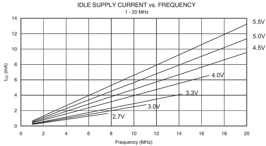
**Figure 127.** Idle Supply Current vs.  $V_{CC}$  (Internal RC Oscillator, 8 MHz)
