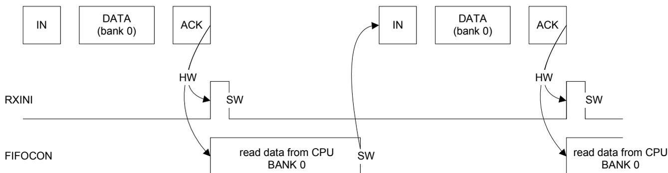
**Figure 30-26.** Example of an IN Pipe with 2 Data Banks
