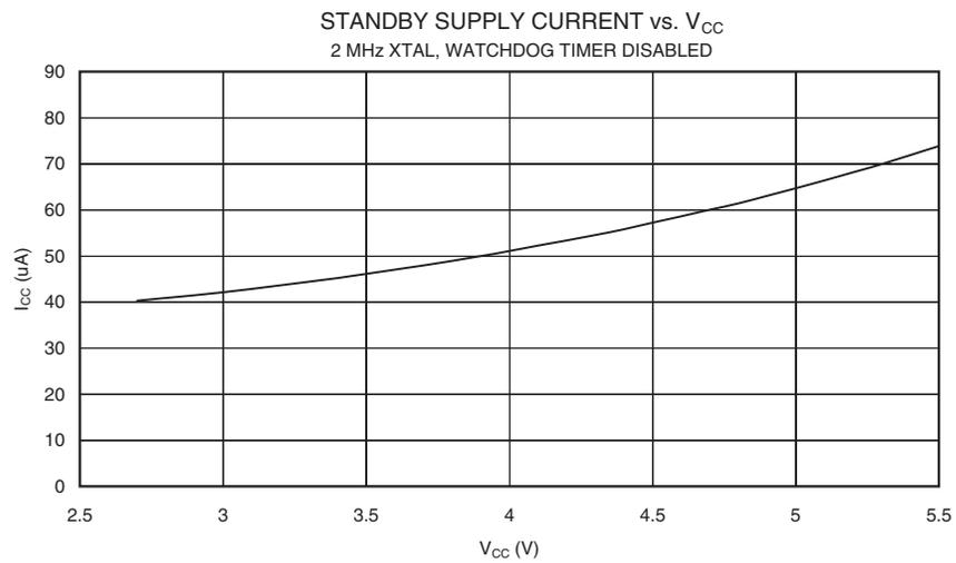
**Figure 139.** Standby Supply Current vs.  $V_{CC}$  (4 MHz Resonator, Watchdog Timer Disabled)
