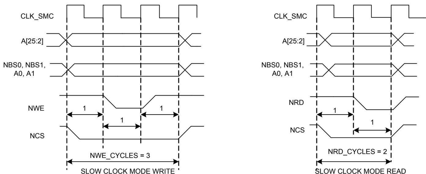
**Table 27-4.** Read and Write Timing Parameters in Slow Clock Mode
