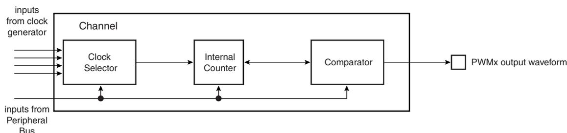
Each of the 7 channels is composed of three blocks:
