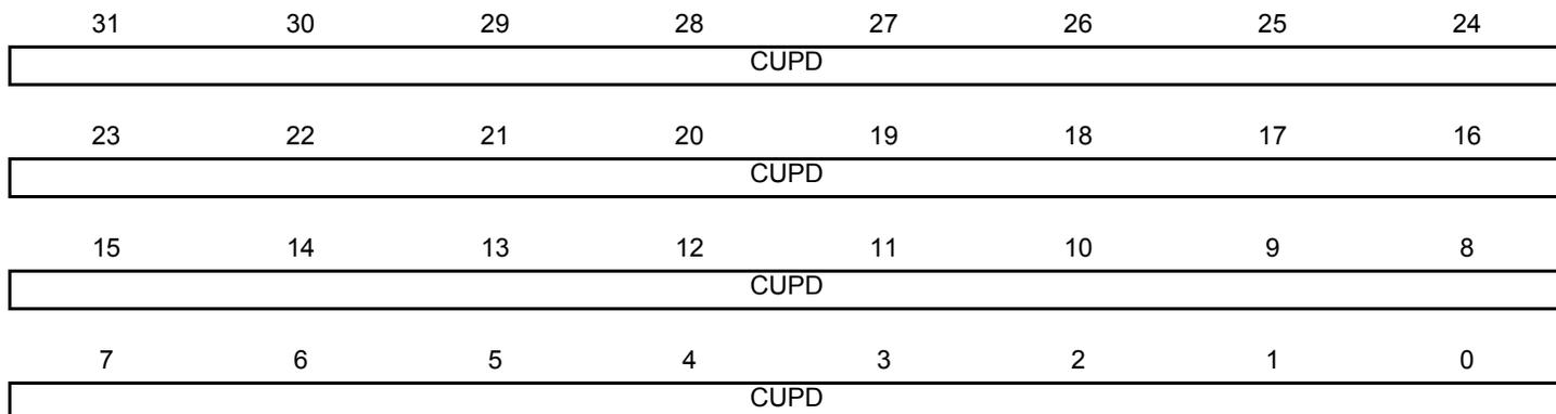
This register acts as a double buffer for the period or the duty cycle. This prevents an unexpected waveform when modifying the waveform period or duty-cycle.
