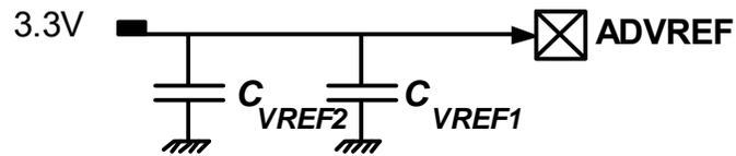
Refer to [Section 38.4 on page 765](#) for decoupling capacitors values and electrical characteristics.
