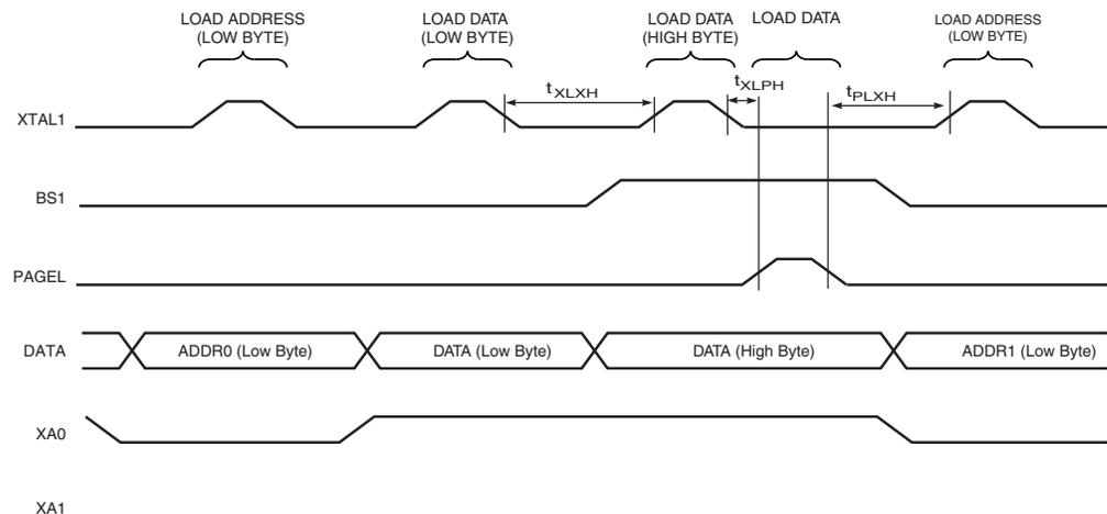
Note: 1. The timing requirements shown in Figure 109 (i.e.,  $t_{DVXH}$ ,  $t_{XHXL}$ , and  $t_{XLDX}$ ) also apply to loading operation.
