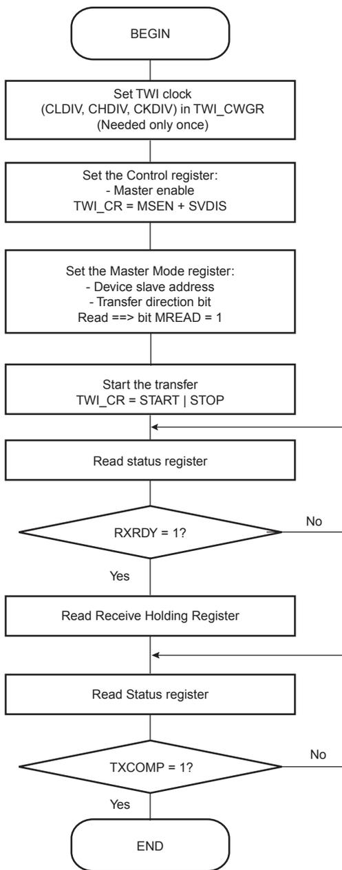
Figure 24-17. TWI Read Operation with Single Data Byte and Internal Address
