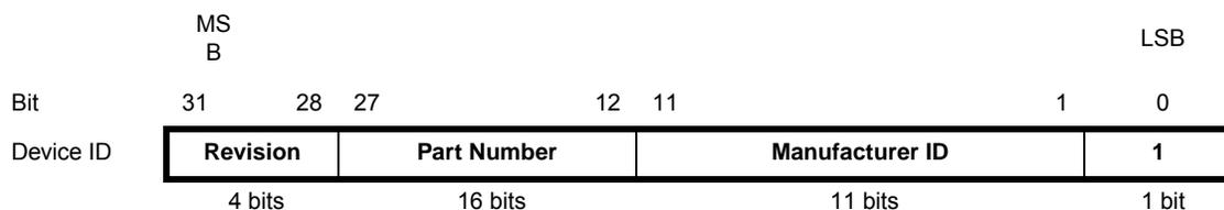
**Revision** This is a 4 bit number identifying the revision of the component. Rev A = 0x0, B = 0x1, etc.
