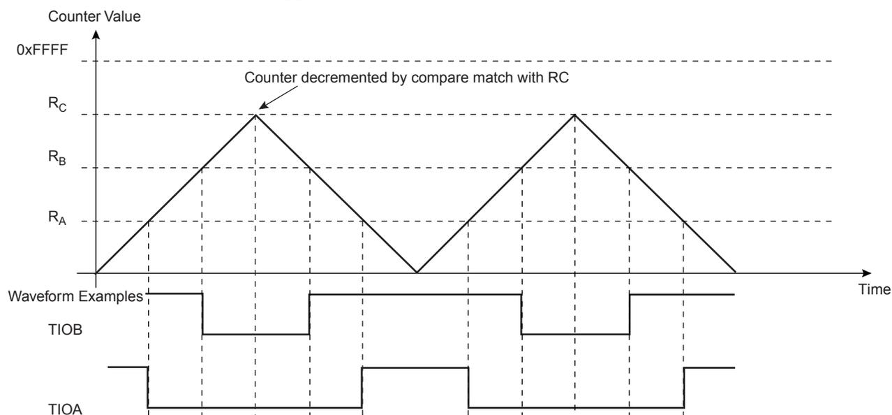
**Figure 31-13. WAVSEL = 11 With Trigger**
