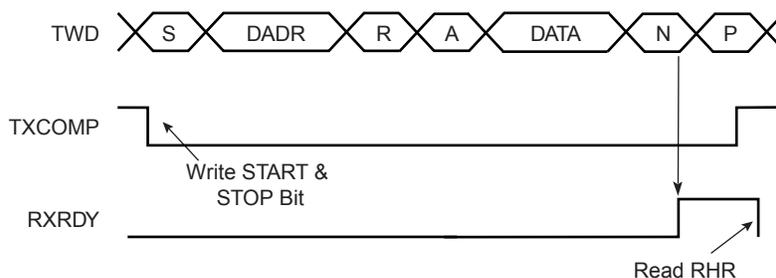
**Figure 24-10.** Master Read with Multiple Data Bytes
