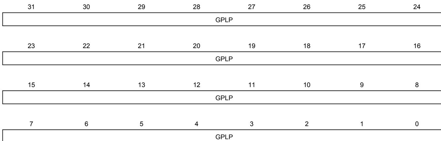
These registers are general purpose 32-bit registers that are reset only by power-on-reset. Any other reset will keep the content of these registers untouched.
