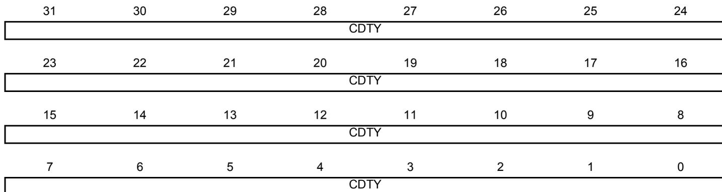
Only the first 20 bits (internal channel counter size) are significant.
