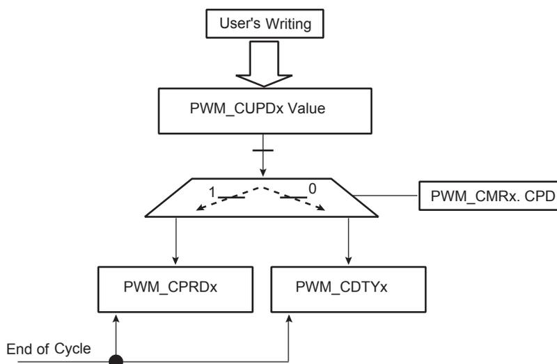
To prevent overwriting the CUPDx by software, the user can use status events in order to synchronize his software. Two methods are possible. In both, the user must enable the dedicated interrupt in IER at PWM Controller level.
