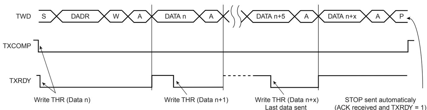
**Figure 24-8. Master Write with One Byte Internal Address and Multiple Data Bytes**
