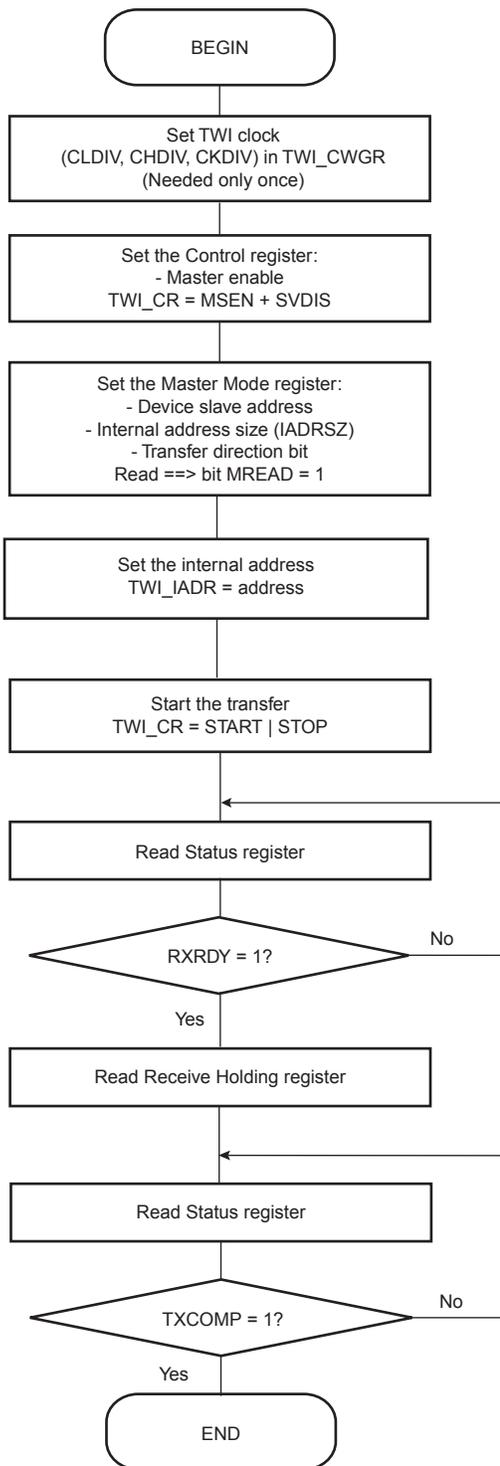
Figure 24-18. TWI Read Operation with Multiple Data Bytes with or without Internal Address
