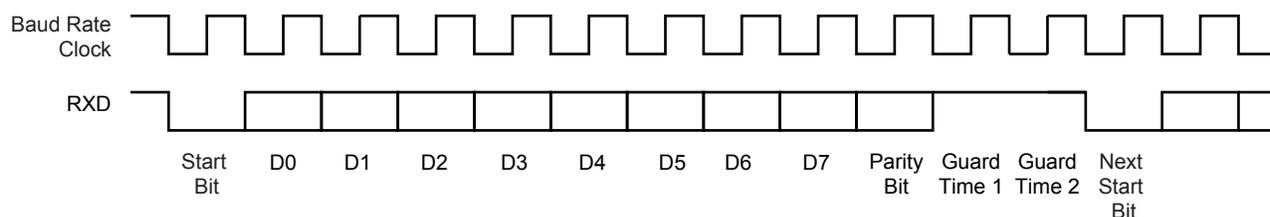
**Figure 26-32.** T = 0 Protocol with Parity Error
