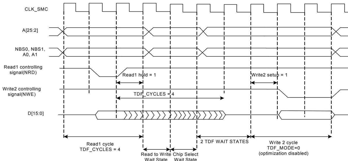
**Figure 27-26.** TDF Mode = 0: TDF wait states between read and write accesses on the same chip select.
