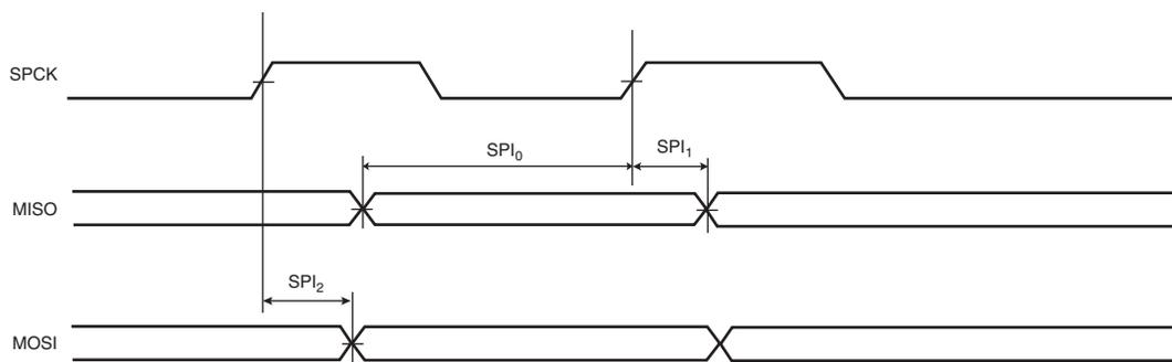
**Figure 38-7.** SPI Master mode with (CPOL=0 and NCPHA=1) or (CPOL=1 and NCPHA=0)
