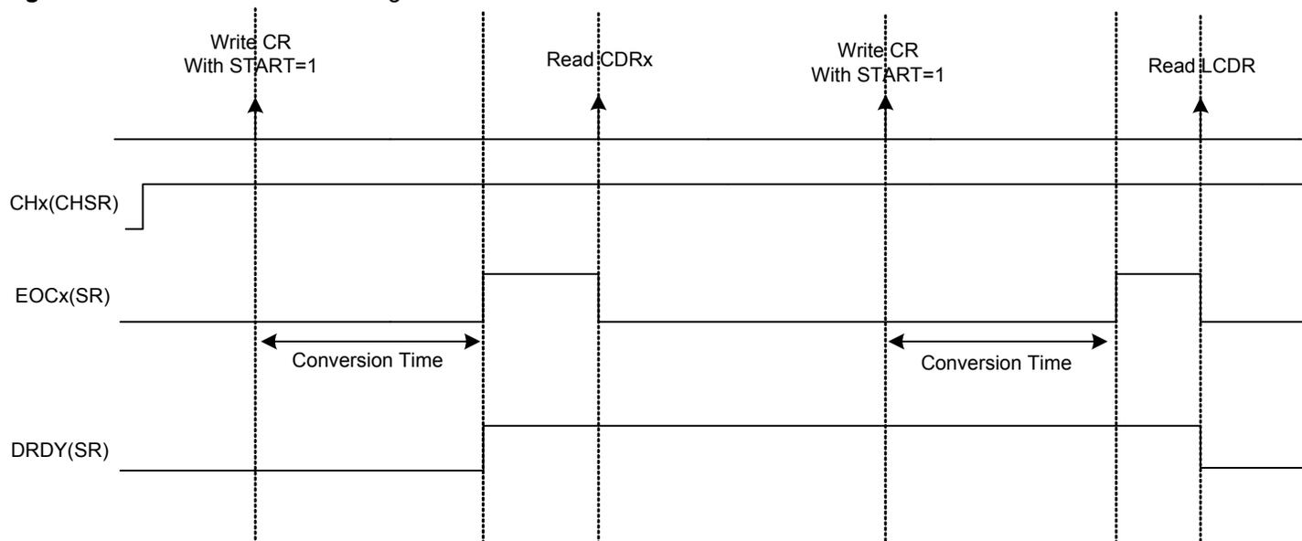
If the CDR is not read before further incoming data is converted, the corresponding Overrun Error (OVRE) flag is set in the Status Register (SR).
