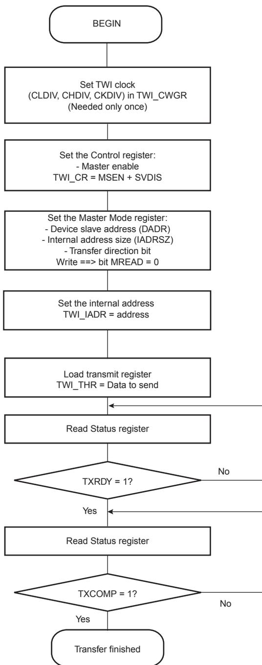
Figure 24-15. TWI Write Operation with Multiple Data Bytes with or without Internal Address
