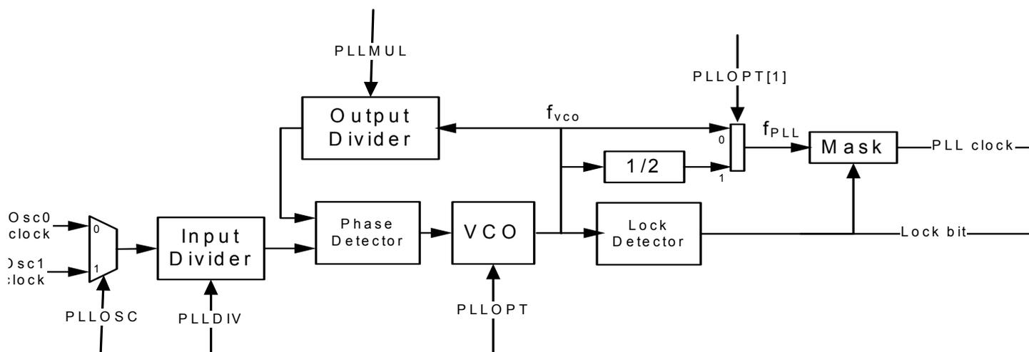
**Figure 13-3.** PLL with control logic and filters
