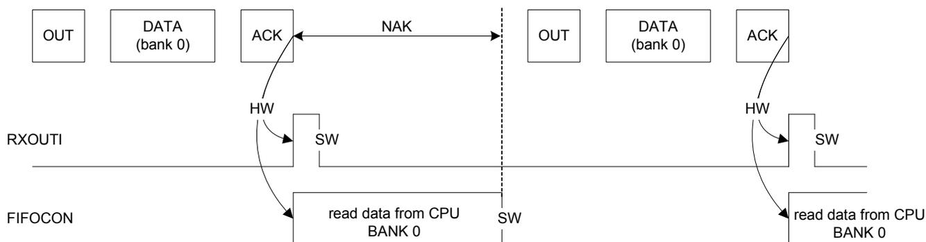
**Figure 30-21.** Example of an OUT Endpoint with 2 Data Banks
