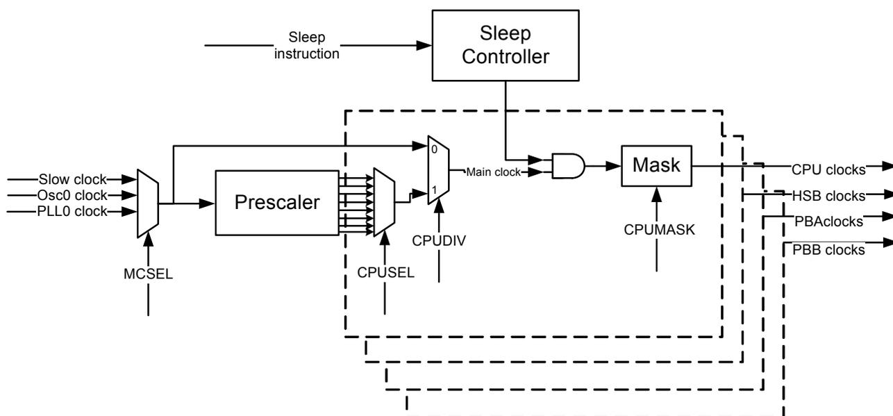
**Figure 13-4.** Synchronous clock generation
