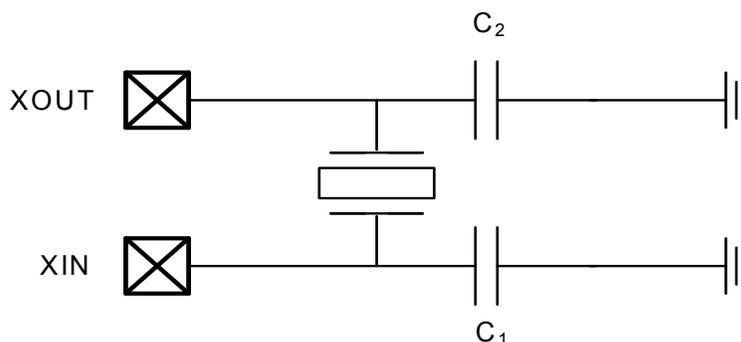
**Figure 13-2.** Oscillator connections
