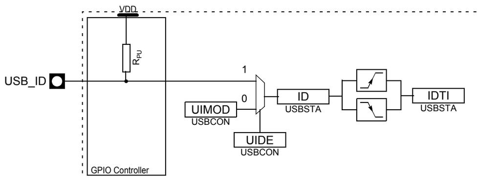
The USB mode (device or host) can be either detected from the USB\_ID pin or software selected from the UIMOD bit, according to the UIDE bit. This allows the USB\_ID pin to be used as a general purpose I/O pin even when the USB interface is enabled.
