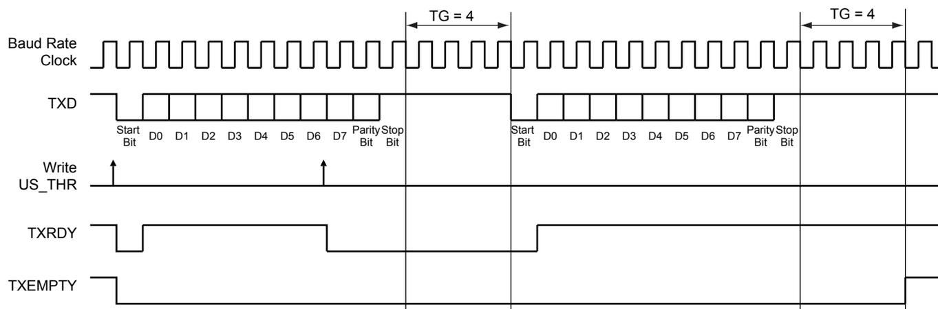
Table 26-7 on page 322 indicates the maximum length of a timeguard period that the transmitter can handle in relation to the function of the Baud Rate.
