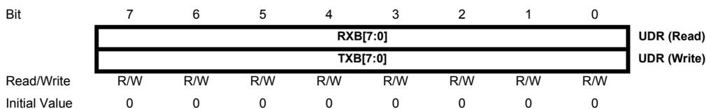
The USART Transmit Data Buffer Register and USART Receive Data Buffer Registers share the same I/O address referred to as USART Data Register or UDR. The Transmit Data Buffer Register (TXB) will be the destination for data written to the UDR Register location. Reading the UDR Register location will return the contents of the Receive Data Buffer Register (RXB).
