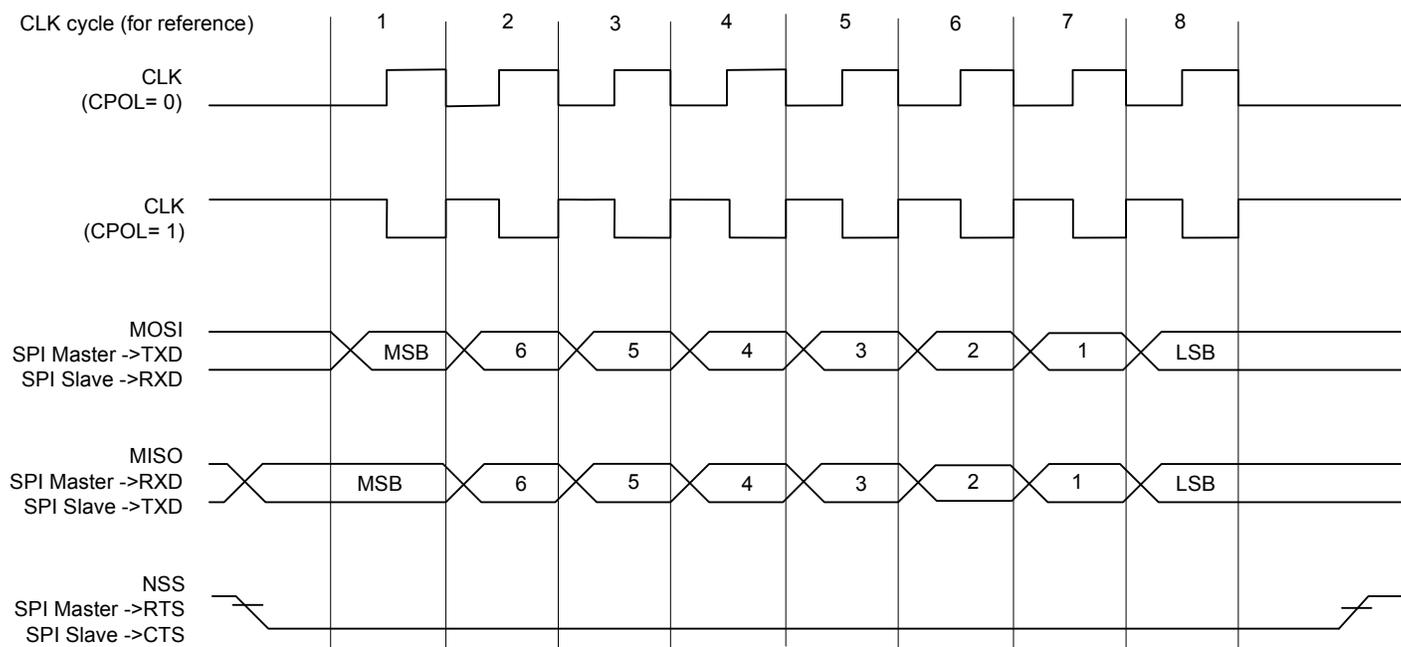
**Figure 26-39.** SPI Transfer Format (CPHA=0, 8 bits per transfer)
