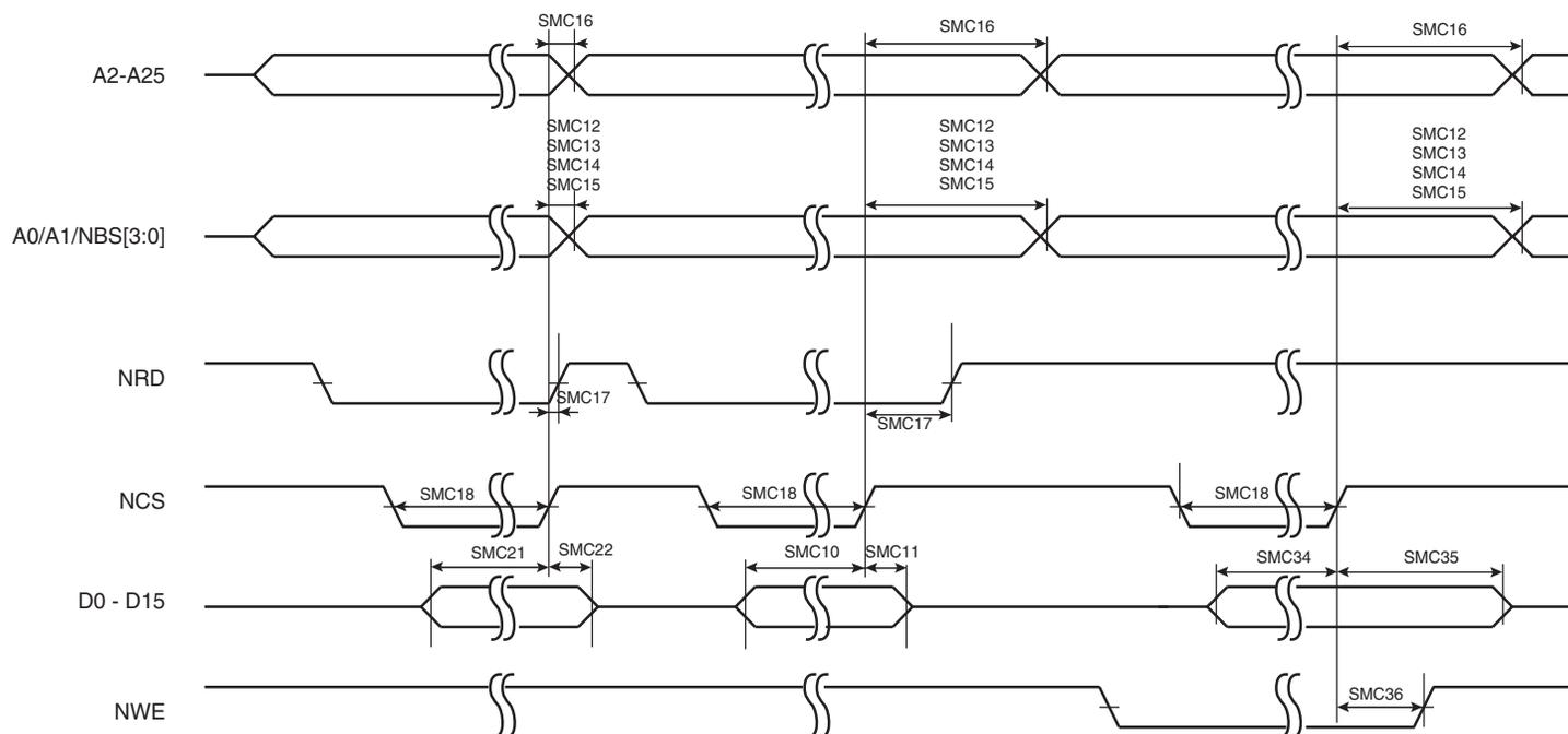
**Figure 38-3.** SMC Signals for NRD and NRW Controlled Accesses.
