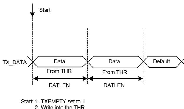
Note: 1. STTDLY is set to 0. In this example, THR is loaded twice. FSDEN value has no effect on the transmission. SyncData cannot be output in continuous mode.
